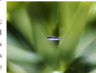
Figure 2: Rod shaped metallic inclusion
